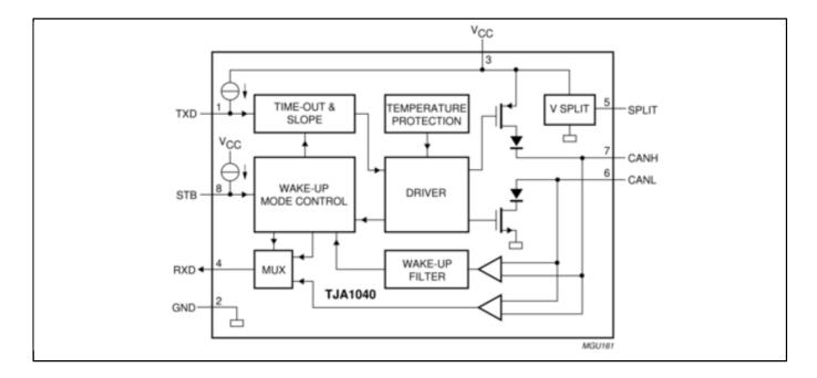
View additional information for High-Speed CAN Transceiver with Standby Mode.
