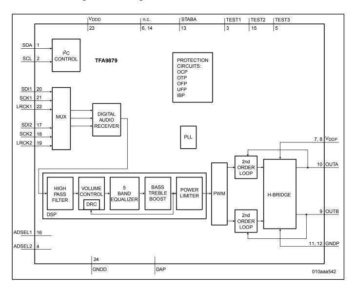
View additional information for TFA9879HN, Mono BTL Class D Audio Amplifier for Portable Applications with Digital Input.
