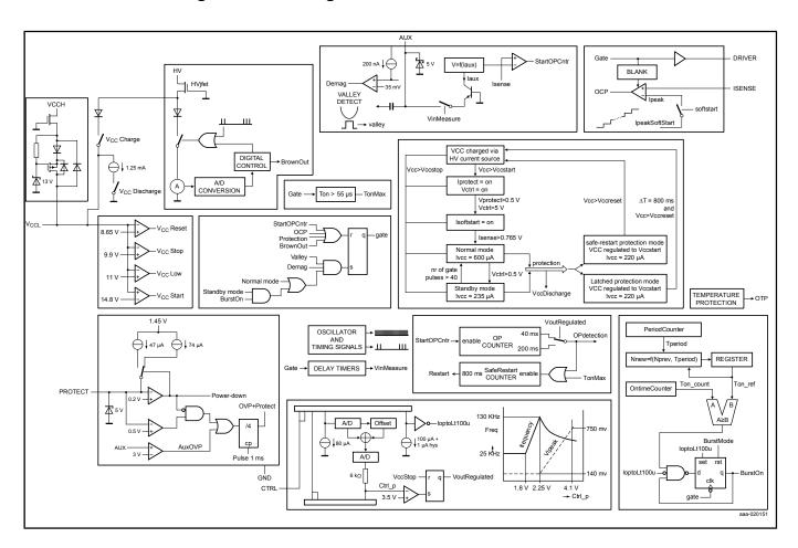
View additional information for GreenChip SMPS Primary Side Control IC with Fixed Frequency Operation.
