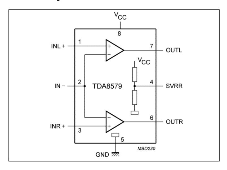
View additional information for Dual Common-mode Rejection Differential Line Receiver.
