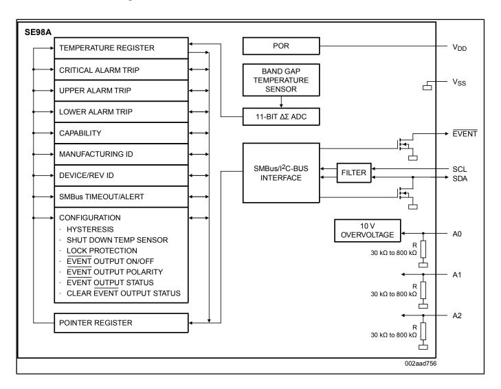
View additional information for DDR Memory Module Temp Sensor, 1.7 V to 3.6 V.
