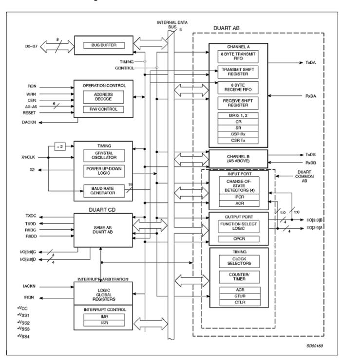
View additional information for Quad Universal Asynchronous Receiver/Transmitter (QUART).
