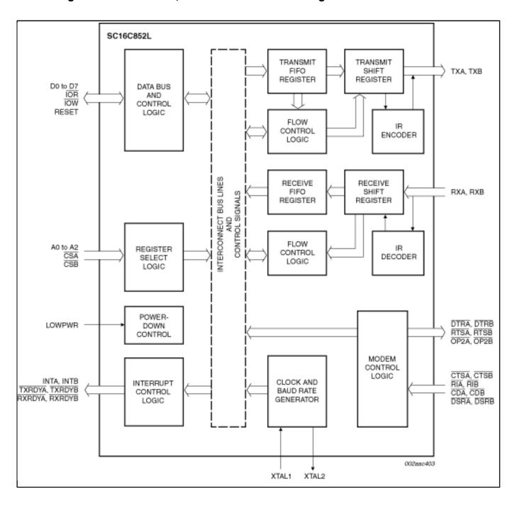
View additional information for 1.8 V dual UART, 5 Mbit/s (max.) with 128-byte FIFOs, infrared (IrDA) and 16 mode or 68 mode bus interface.
