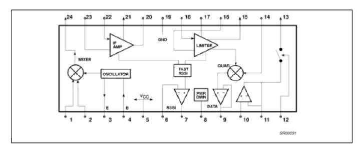
View additional information for Low-Voltage Mixer FM IF System with Filter Amplifier and Data Switch.
