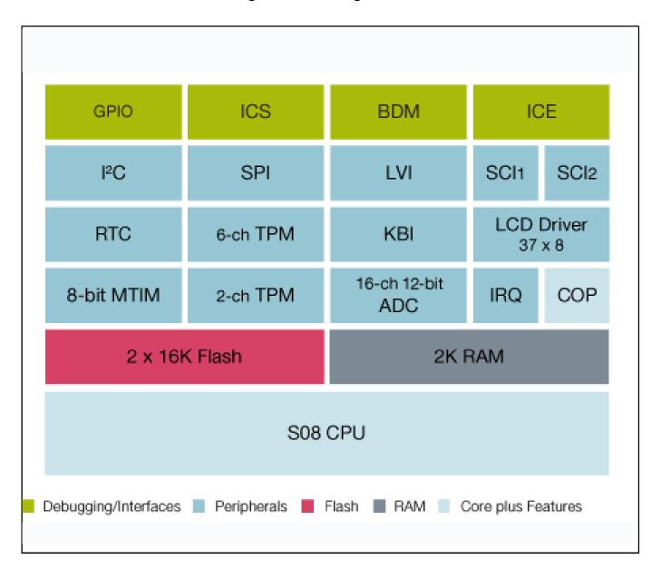
**S08LG32 Instrument Cluster Block Diagram**
