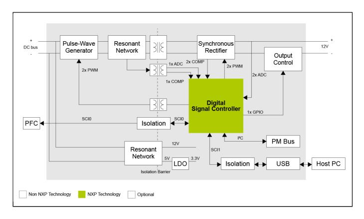
View additional information for LLC Resonant Converter with Sync Rectifier.
