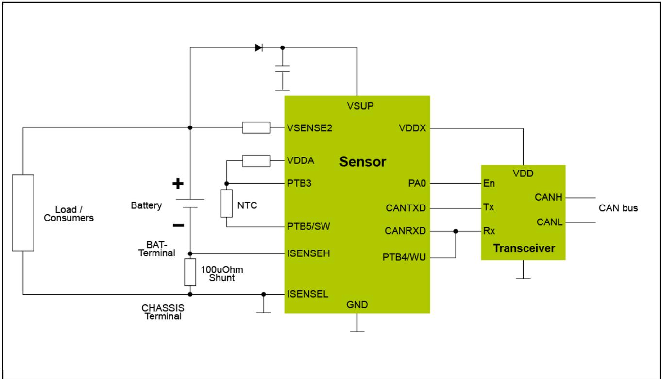
View additional information for [12 V Lead-Acid Battery Sensor with CAN](#).
