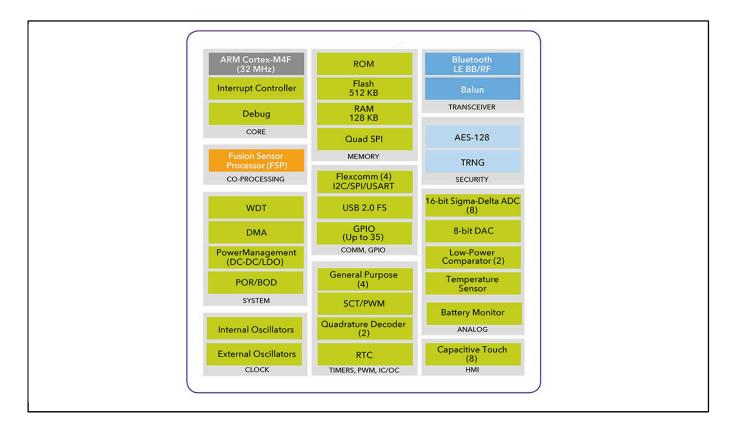
View additional information for QN908x: Ultra-Low-Power Bluetooth Low Energy System on Chip Solution.
