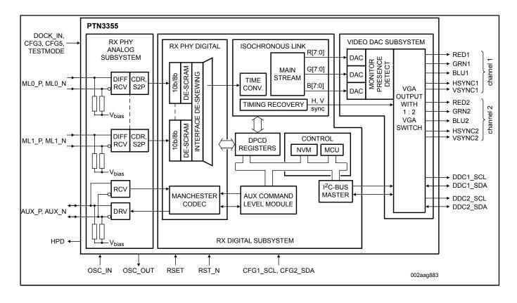
View additional information for Low Power DisplayPort to VGA Adapter with Integrated 1-2 VGA Switch.
