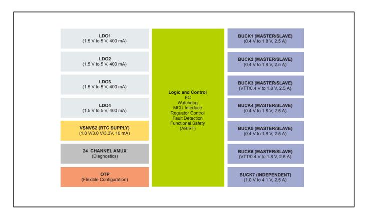
View additional information for 12-Channel Power Management Integrated Circuit (PMIC) for High-Performance Processing Applications.
