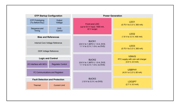
View additional information for Power Management Integrated Circuit (PMIC) for Low Power Application Processors.
