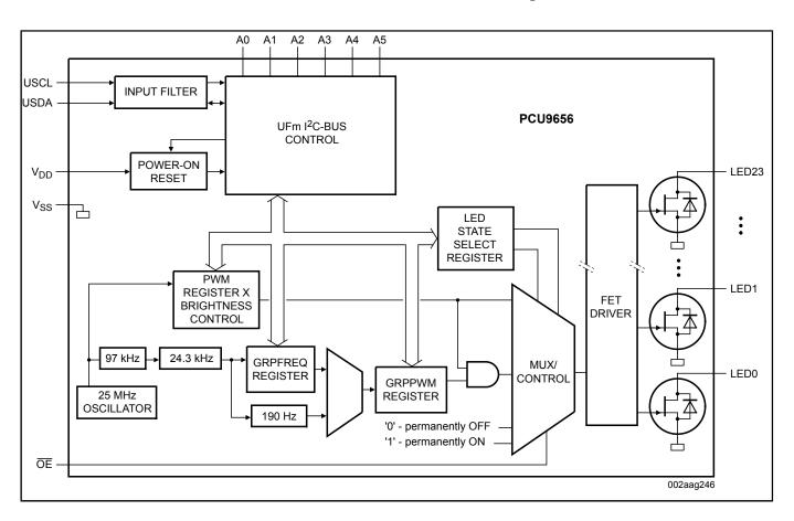
View additional information for 24-Bit UFm 5 MHz I<sup>2</sup>C-Bus 100 MA 40 V LED Driver.
