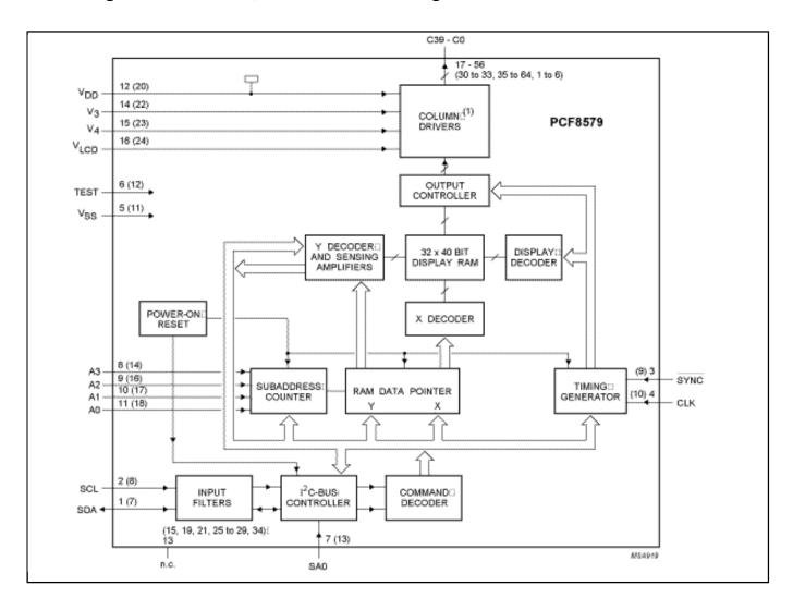
View additional information for LCD Column Driver for Dot Matrix Graphic Displays.
