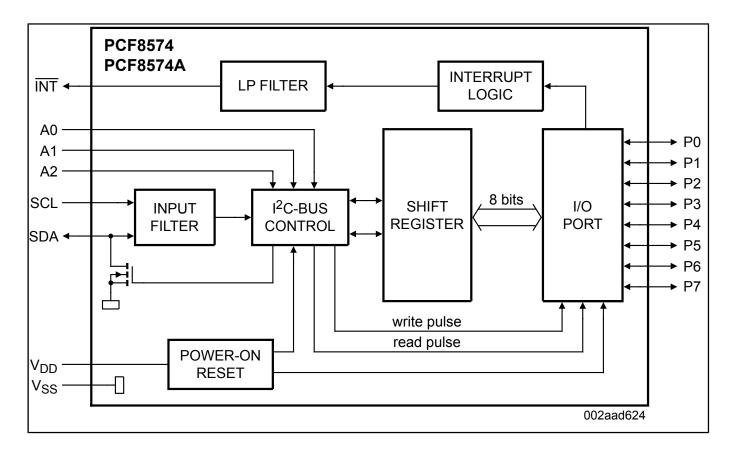
View additional information for Remote 8-Bit I/O Expander for I<sup>2</sup>C#Bus with Interrupt.
