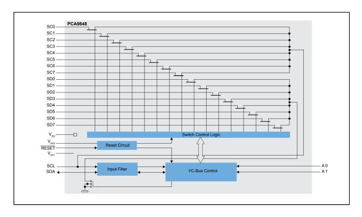
View additional information for Eight-Channel Ultra-Low Voltage, Fm+ I<sup>2</sup>C-Bus Switch with Reset.
