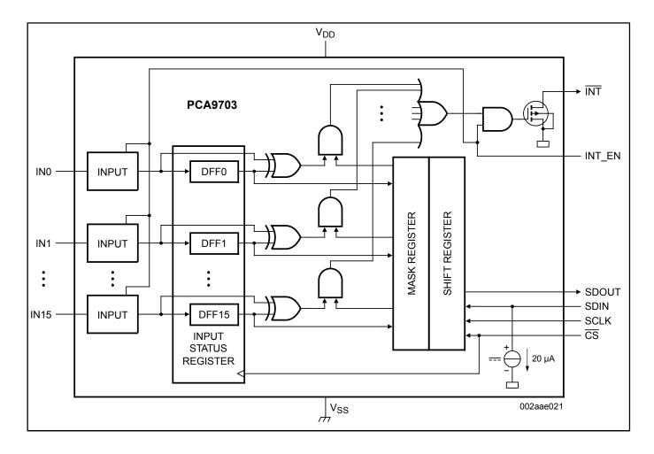
View additional information for 18 V Tolerant SPI 16-Bit GPI with Maskable INT.
