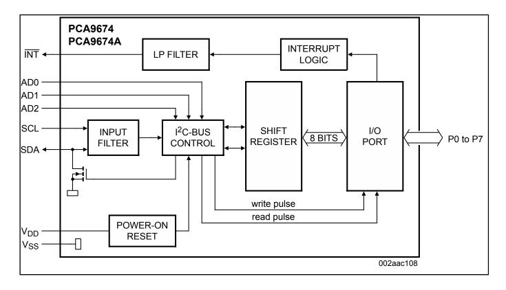
View additional information for Remote 8-Bit I/O Expander for Fm+ I2C-Bus with Interrupt.
