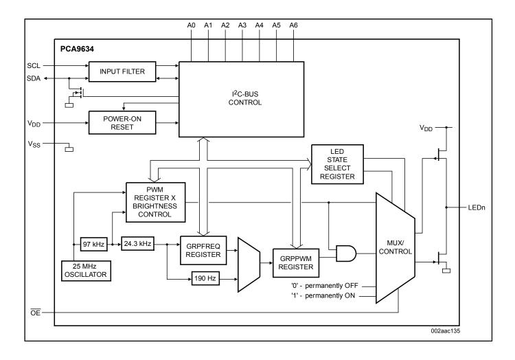
Block diagram: PCA9634BS, PCA9634D, PCA9634PW Block Diagram
