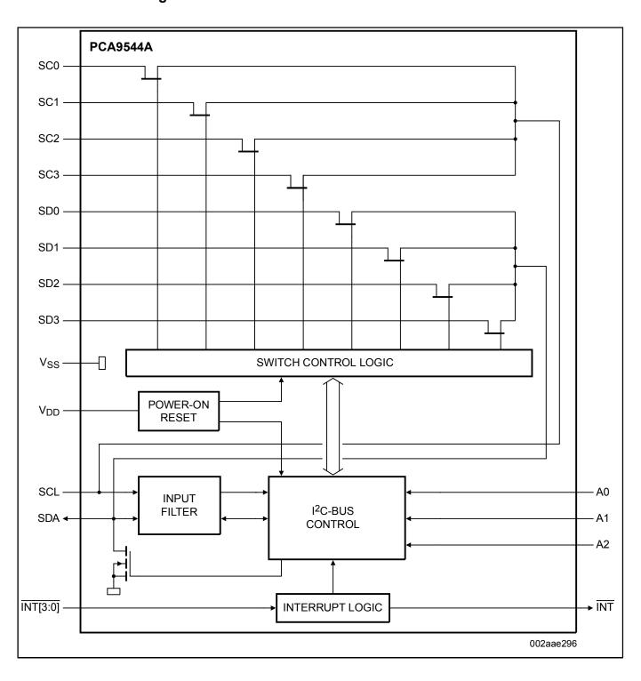
PCA9544ABS, PCA9544AD, PCA9544APW Block Diagram
