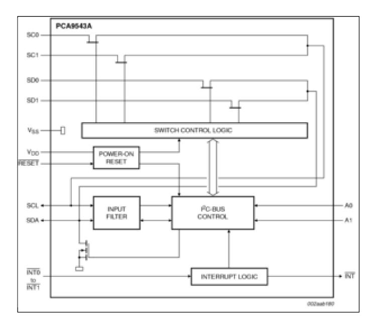
View additional information for Two-Channel I2C-Bus Switch with Interrupt Logic and Reset.
