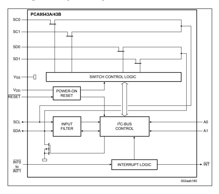
PCA9543AD, PCA9543APW, PCA9543BPW, PCA9543CPW Block Diagram Block Diagram
