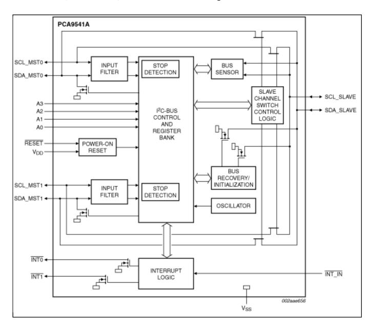
View additional information for 2-1 I2C-Bus Controller Selector with Interrupt Logic and Reset.
