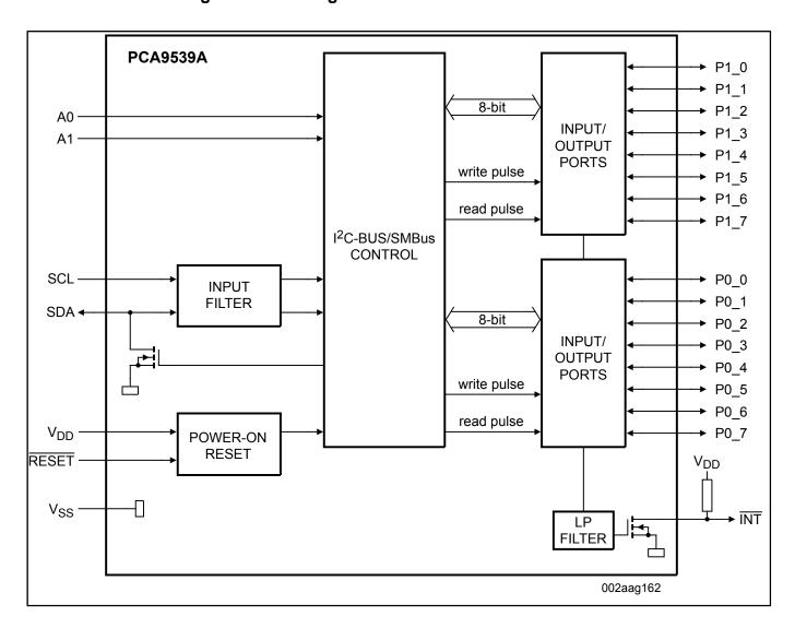
View additional information for Low Voltage 16-Bit I<sup>2</sup>C-Bus I/O Port with Interrupt and Reset.
