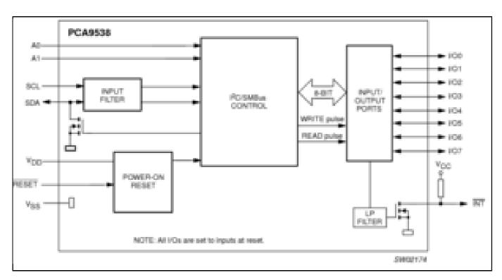
View additional information for 8-Bit I2C-Bus and SMBus Low-Power I/O Port with Interrupt and Reset.
