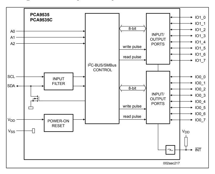
View additional information for 16-Bit I2C-Bus and SMBus, Low-Power I/O Port with Interrupt.
