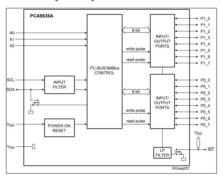
View additional information for Low-Voltage 16-Bit I<sup>2</sup>C-Bus I/O Port with Interrupt.
