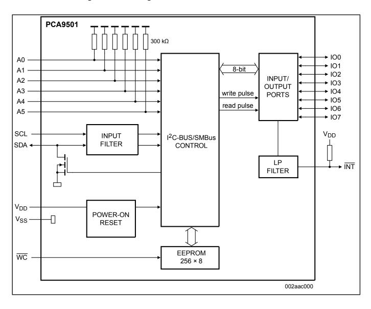
Block diagram: PCA9501BS, PCA9501D, PCA9501PW Block Diagram
