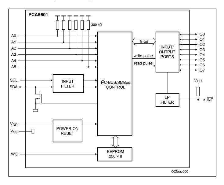
Block diagram: PCA9501BS, PCA9501D, PCA9501PW Block Diagram
