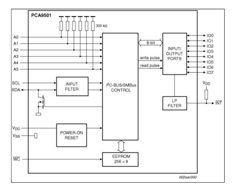
View additional information for 8-Bit I2C-Bus and SMBus I/O Port with Interrupt, 2-Kbit EEPROM and 6 Address Pins.
