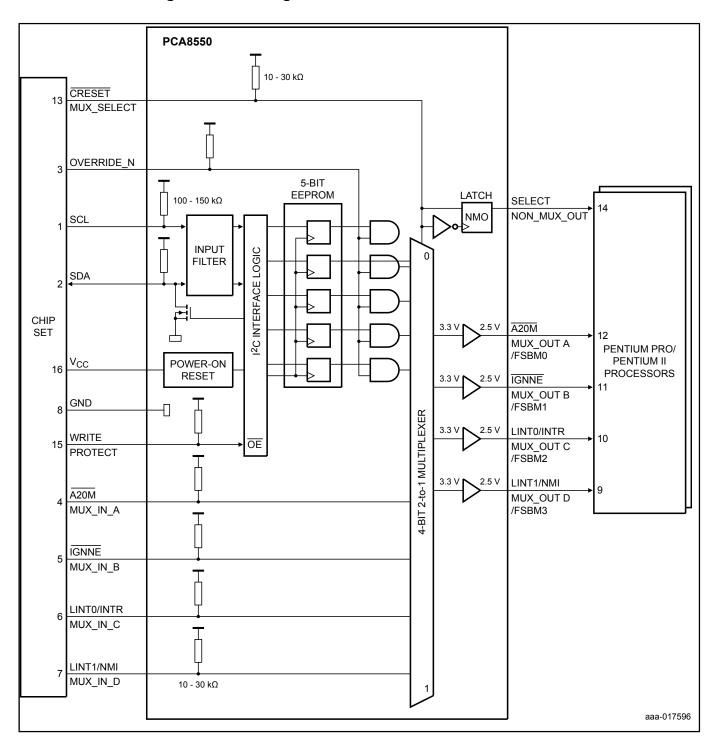
View additional information for 4-Bit Multiplexed/1-Bit Latched 5-Bit I<sup>2</sup>C EEPROM DIP Switch.
