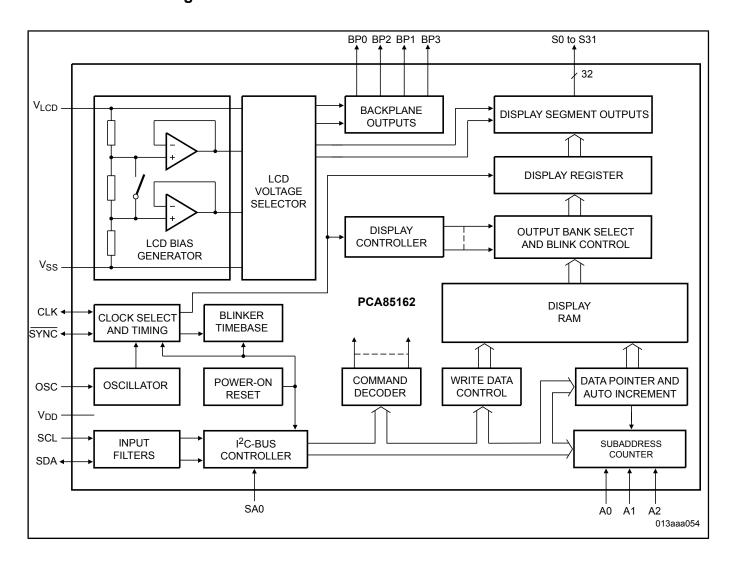
View additional information for 32 X 4 Automotive LCD Driver for Low Multiplex Rates.
