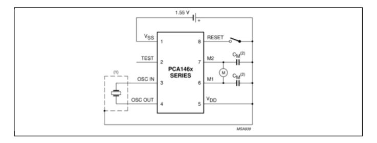
View additional information for 32 KHz Watch Circuits with Adaptive Motor Pulse.
