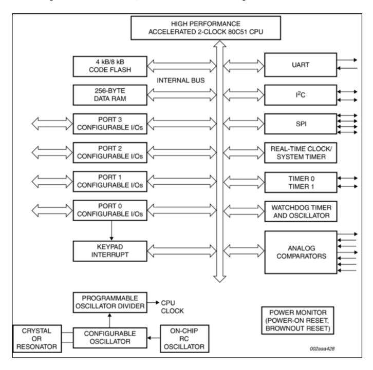
View additional information for 8-Bit Microcontrollers with Accelerated Two Clock 80C51 Core 4 KB/8 KB 3 V Low-Power Flash with 8-Bit A/D Converter.
