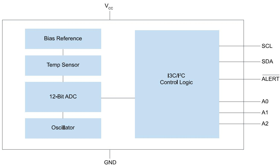
View additional information for I3C/I<sup>2</sup>Cバス対応、±0.5°C精度デジタル温度センサ.
