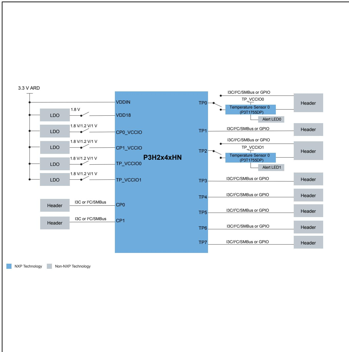
View additional information for [P3H2x4xHN I<sup>2</sup>CハブArduino®シールド評価ボード](#).
