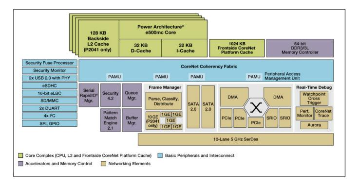
View additional information for QorlQ® P2040/P2041 Multicore Communications Processors with Data Path.
