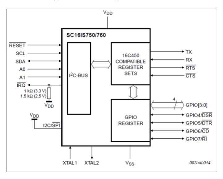
View additional information for SC16IS750 SPI/I<sup>2</sup>C to UART Bridge Demo Board.
