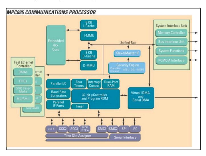
View additional information for PowerQUICC® Processor with CPM with ATM, USB, Dual 10/100 Ethernet, Security.
