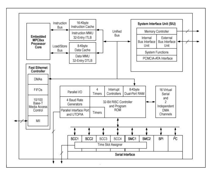
View additional information for PowerQUICC® Processor with CPM (4 SCC, 2 SMC), 10/100 Ethernet.
