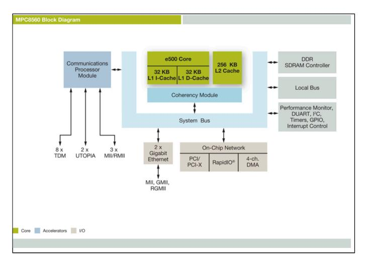
View additional information for PowerQUICC® III Processor with TDM, DDR, PCI, PCIx Express®, RapidIO, 1 GB Ethernet, Security, CPM with UTOPIA.
