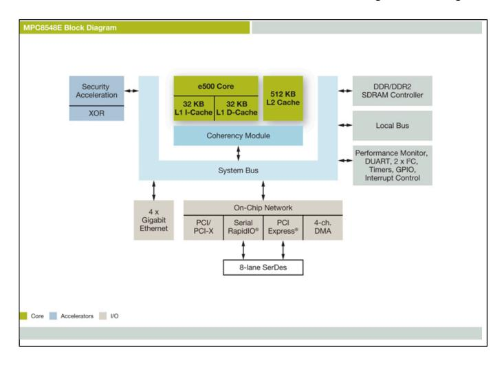
View additional information for PowerQUICC® III Processor with DDR2, PCI, PCI Express®, Serial RapidIO, SerDes, 1 GB Ethernet, Security.
