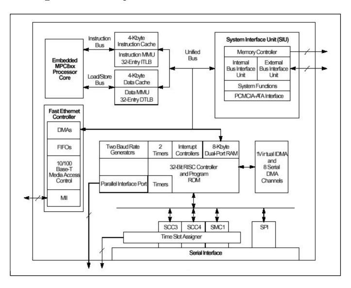
View additional information for PowerQUICC® Processor with CPM (2 SCC, 1 SMC), 10/100 Ethernet.
