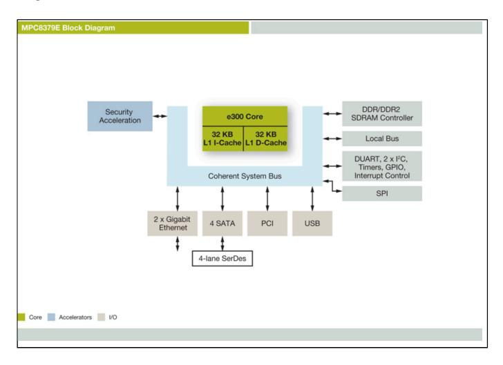
View additional information for PowerQUICC® II Pro Processor with DDR2, PCI, PCI Express, SATA, 1 GB Ethernet, USB, Security.
