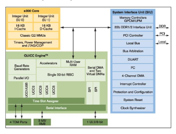
View additional information for Low-Power PowerQUICC® II Pro Processor with DDR2, TDM, PCI, Security, USB, QUICC Engine® with UTOPIA.
