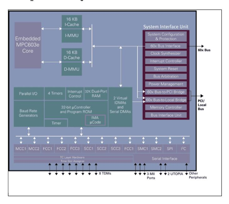
View additional information for PowerQUICC® II Processor with 256-ch. HDLC, UTOPIA II, 10/100 Ethernet.
