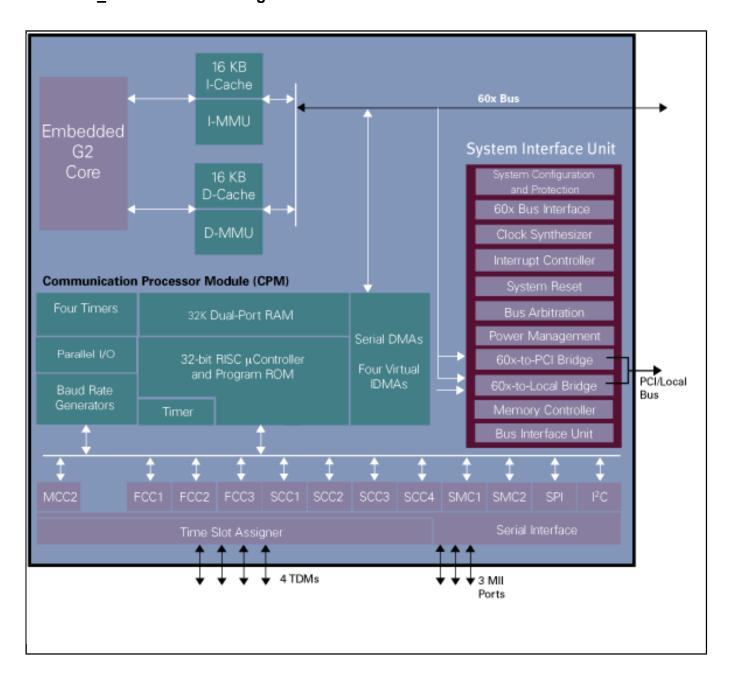
View additional information for PowerQUICC® II Processor with PCI, 128-ch. HDLC, 10/100 Ethernet.
