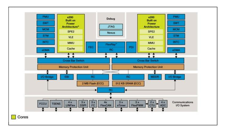
View additional information for Ultra-Reliable MPC567xK MCU for Automotive and Industrial Radar Applications.
