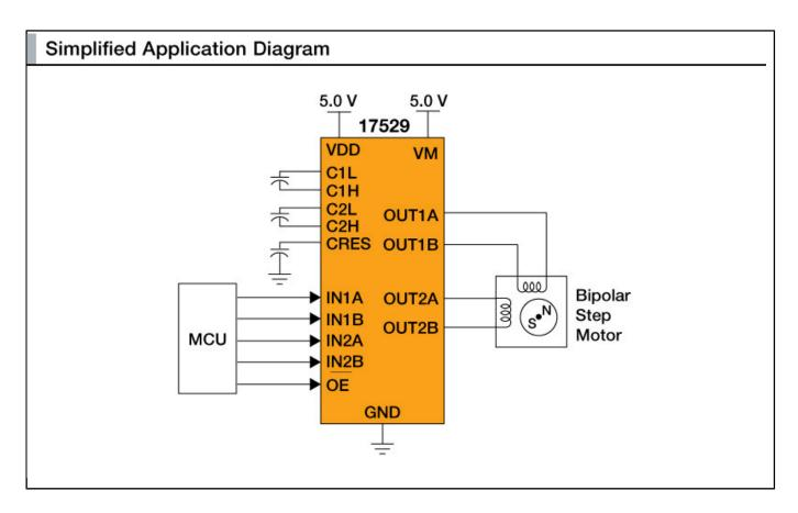
View additional information for Dual H-Bridge, Motor Driver, 2-6.8 V, 1.4 A, 200 kHz.
