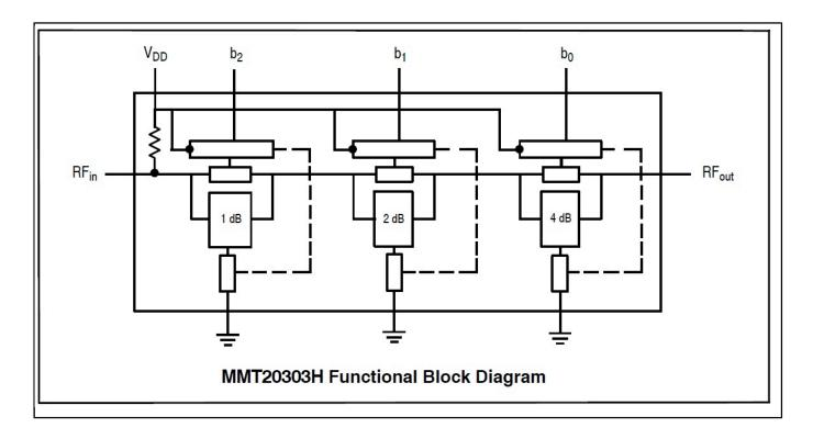
View additional information for 50-4000 MHz, 3-Bit 1 dB LSB Digital Step Attenuator.
